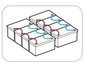
Connect the batteries in parallel.
