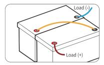
After series connection, the voltage of the battery system will be doubled according to the number of batteries you connect.
