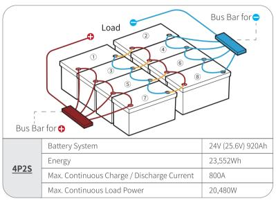
① As  $\bigcirc$  of ① / ③ / ⑤ / ⑦ is connected in series with  $\bigcirc$  of ② / ④ / ⑥ / ⑧, please do not connect  $\bigcirc$  of ① / ③ / ⑤ / ① with  $\bigcirc$  of load or  $\bigcirc$  of ② / ④ / ⑥ / ⑧ with  $\bigcirc$  of load, otherwise the battery system will fail to connect in series
